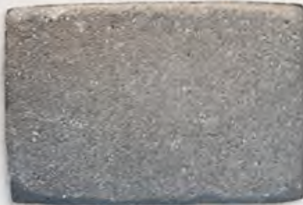
BELGARD COLORGARD PAVER AFTER 15 YEARS OF EXPOSURE
